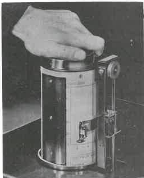
Fig. 2.6 Correct Way to Rotate Drum Manually
