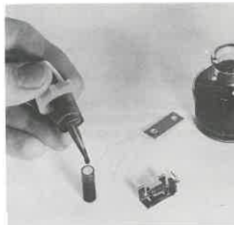
Fig. 2.3 Filling Pen Reservoir
