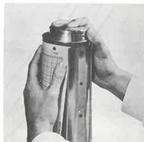
Fig. 2.5 Securing End of Chart Paper
